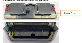
8. While pressing Cover Taken & Cover Front down, reassemble (Red circle). \* Be careful that the Wire does not get stuck.
