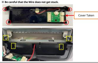
7. Reassemble the Cover Front Hook (Red Circle parts) into the Printer (Yellow ※ Be careful that the Wire does not get stuck.
